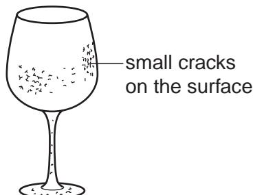
The cracks are caused by differences in the rate of diffusion of sodium ions and hydrogen ions in the glass.
